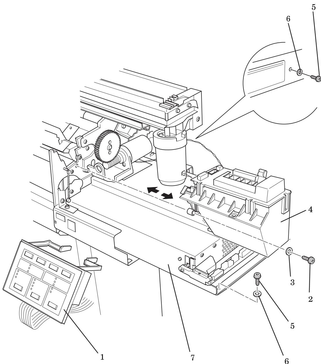
**Figure 5 - Front Panel, Spittoon and Electronics Module**
