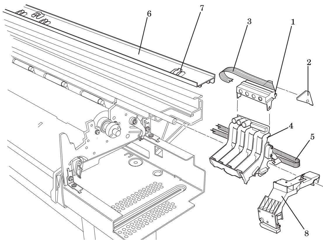
**Figure 8 - Carriage Assembly and Trailing Cable**
