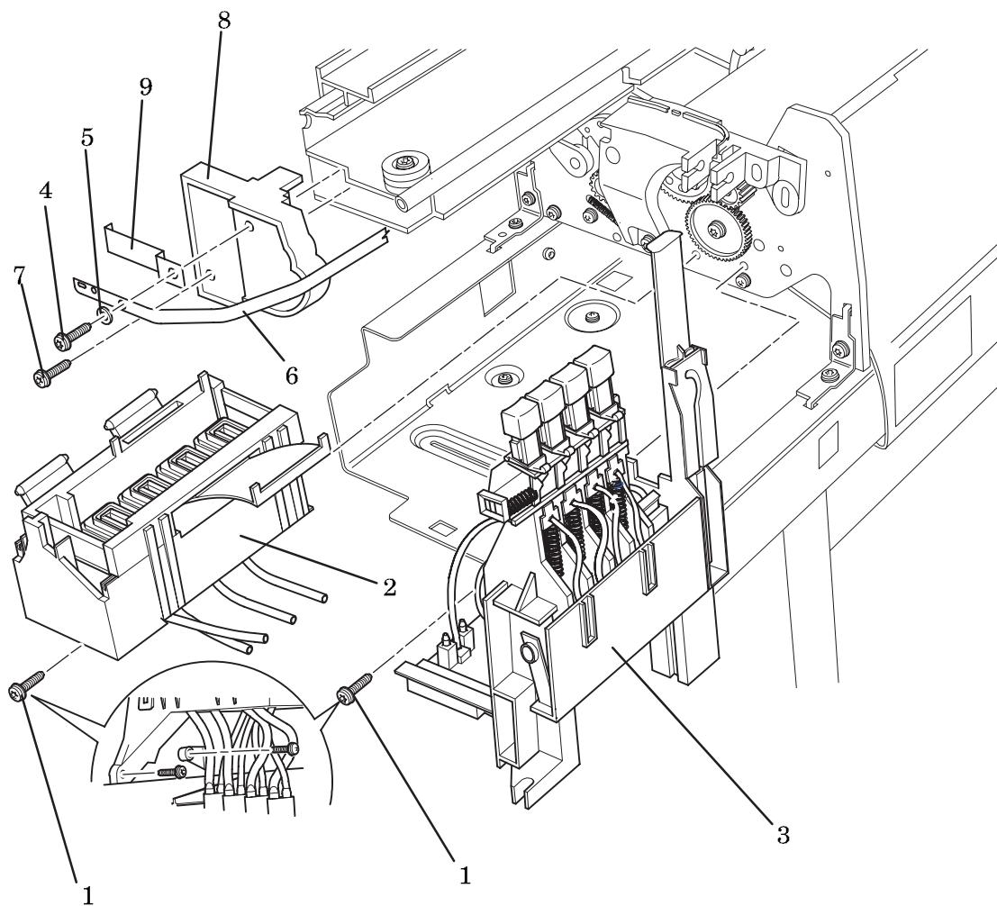
**Figure 7 - Primer Assembly and Service Station Assembly**
