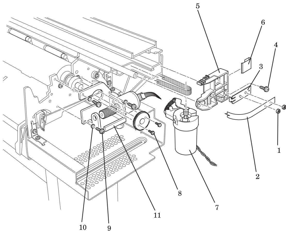
**Fig 6 - X and Y axis Motors and Encoder Strip**
