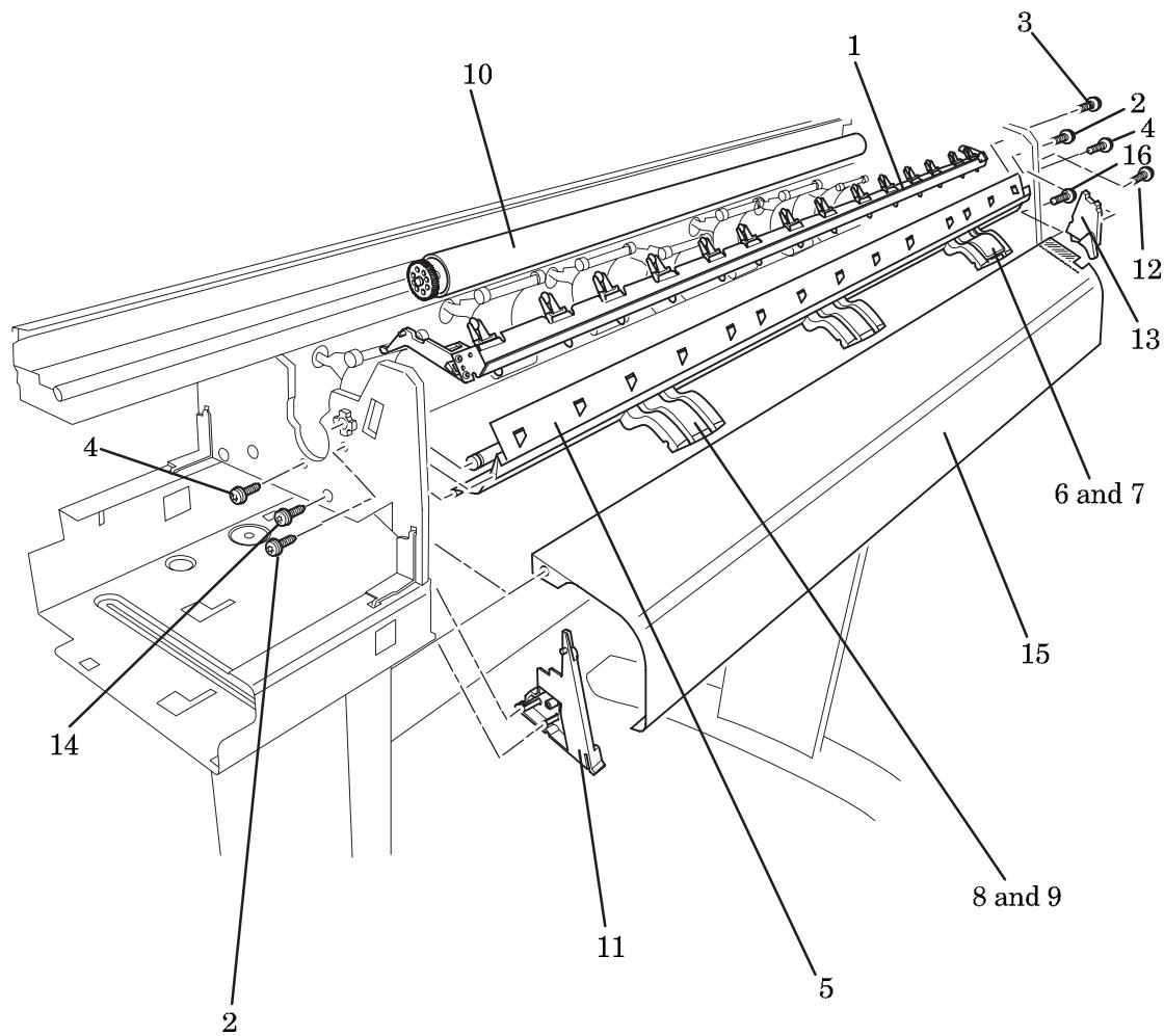
**Figure 11 - Entry Platen, Drive Roller, Bail and Overdrive Assembly**
