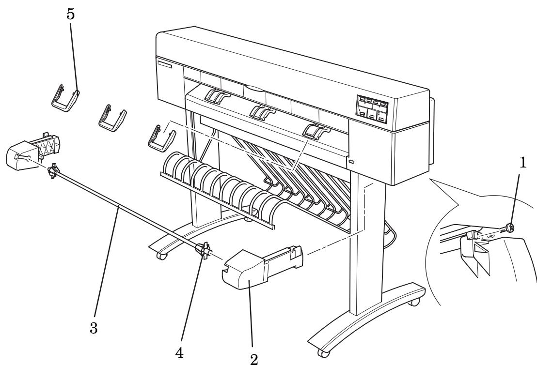
**Figure 3 - Rollfeed Assembly**
