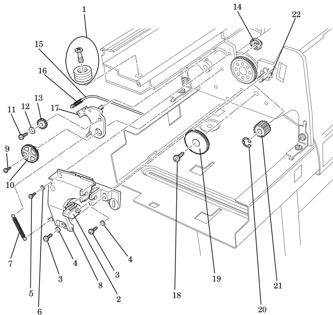
**Figure 9 - Bail and Overdrive Mechanisms**
